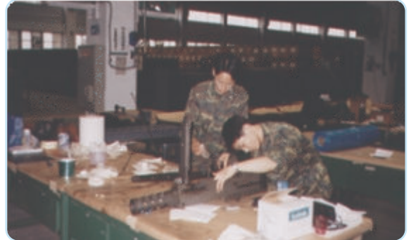
Cleaning and preparation of 0.5 caliber Brownings with Vapro 818 CLP before preservation.
