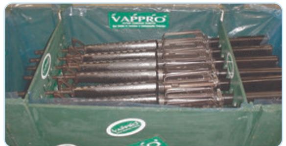
Cleaning and preservation of M16s using Vapro 818 CLP.
