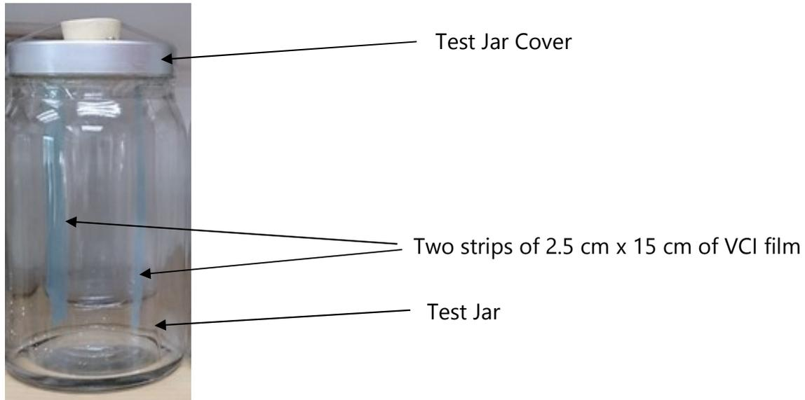
For blank sample, test jar was sealed without inserting two strips of test samples. It had no VCI chemicals and it is only used as a control/ yardstick for the experiment. Please see below picture.
