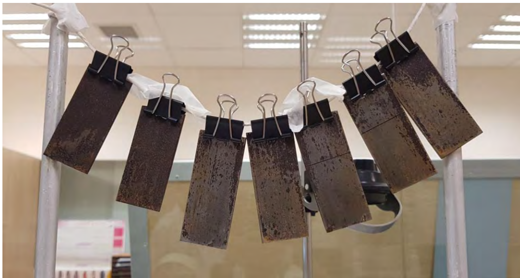
Figure 4: Hanging of metal specimens after soaking in NaCl solution
